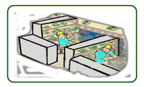
**Unification:** Even if a flowing line cannot be formed, odd operations can be combined together in a place into an operator's work
