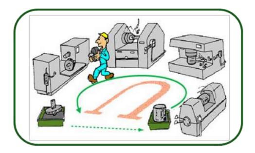
**In-lining:** Is a way to make the production lines simple and effective by integrating the parts processing into the main line in the unit production.
